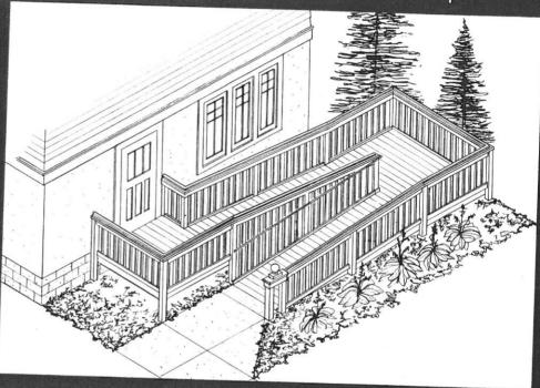
4' wide ramp, with intermediate 6' x 9' landing, and top landing of 6' x 6'.
